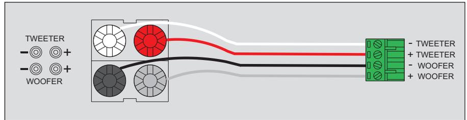
Figure 7. Correct loudspeaker cable polarity.
