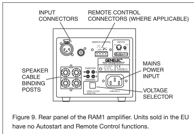
Figure 9. Rear panel of the RAM1 amplifier. Units sold in the EU have no Autostart and Remote Control functions.
