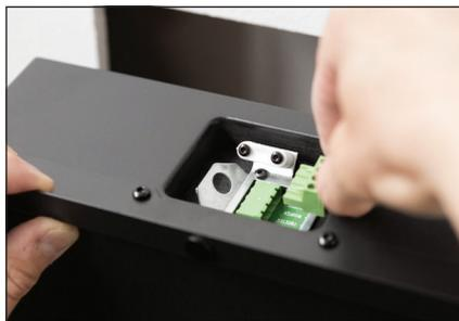
Figure 3. Connect the loudspeaker cable.
