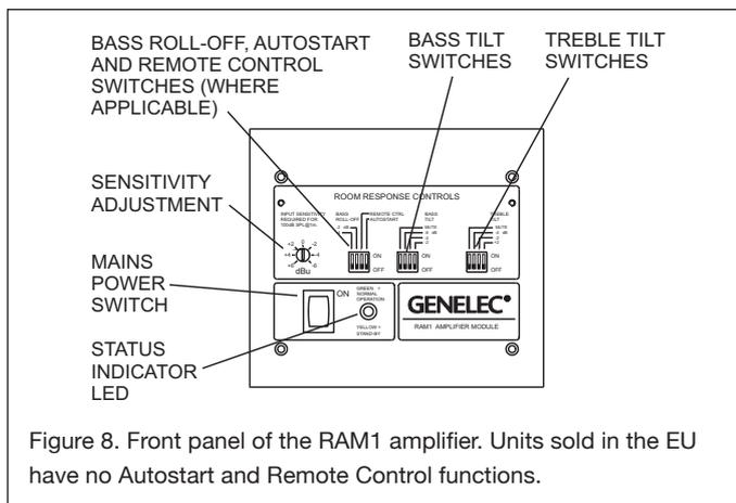
Figure 8. Front panel of the RAM1 amplifier. Units sold in the EU have no Autostart and Remote Control functions.
