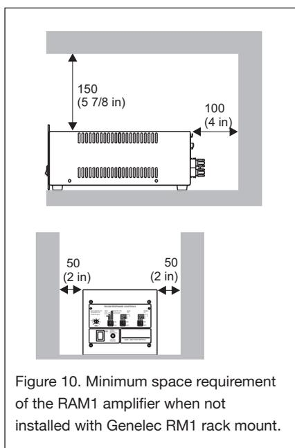
Figure 10. Minimum space requirement of the RAM1 amplifier when not installed with Genelec RM1 rack mount.
